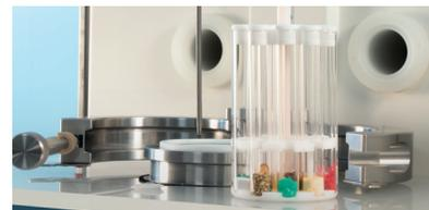
In 2016, the lab switched to Milestone's ultraWAVE Single Reaction Chamber (SRC) microwave system and currently achieves the high quality results and recovery rates it needs for the volatile elements it analyses.
