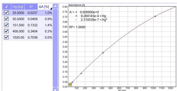
Figure 4 20 ng – 1000 ng Calibration Graph for low to mid-level analysis (ppb, ppm)
