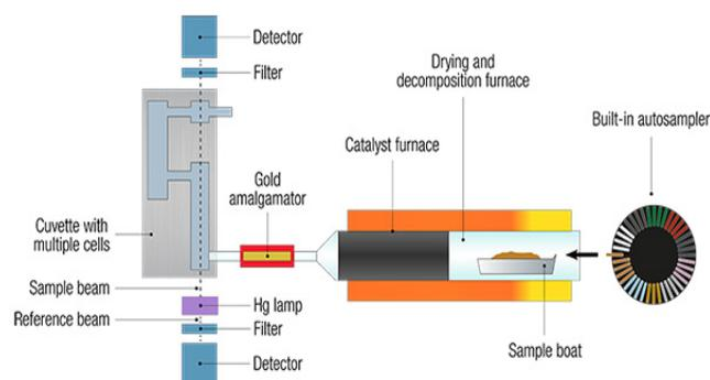
Figure 2 An Internal Schematic of Milestone's DMA-80 *evo*.
