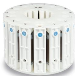
The SK-15 high-pressure and temperature rotor features 15 PTFE-TFM vessels, suitable for digestion of challenging and reactive samples, such as polymers and geological materials.
