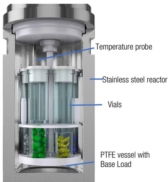
Figure 2 – Schematic of the ultraWAVE's single reaction chamber (SRC)
