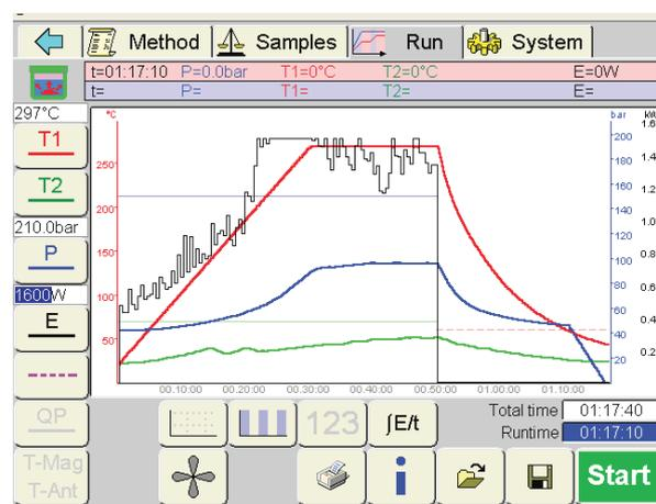
Figure 3 - The ultraWAVE's touch screen controller. The red line is the internal digestion temperature, while the blue line indicates the real-time pressure that is being monitored inside the stainless steel chamber. The black line indicates the microwave power being emitted during the entire digestion cycle.
