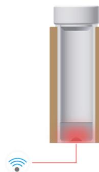
Figure 2 – easyTEMP contactless direct temperature sensor.
