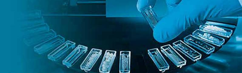
method 7473 for rapid determination of mercury in solids and aqueous samples without sample preparation.
