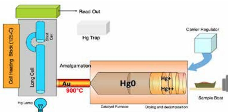
Figure 2. An Internal Schematic of Milestone's DMA-80.
