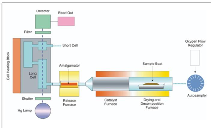
Figure 2. Internal Schematic of Milestone's DMA-80 Direct Mercury Analyzer.
