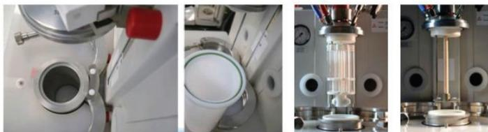
Running parallel reactions using a Microwave-based Reactor.
