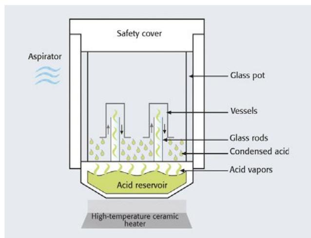
▲ Figure 2. Schematic diagram of the TraceCLEAN.
