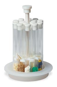
The rack is loaded into the chamber, which is then sealed and pre-pressurized with nitrogen to 40 bar prior to microwave heating. Pre-pressurization prevents splashing or boiling of the sample solutions, avoiding cross contamination or loss of volatiles.
